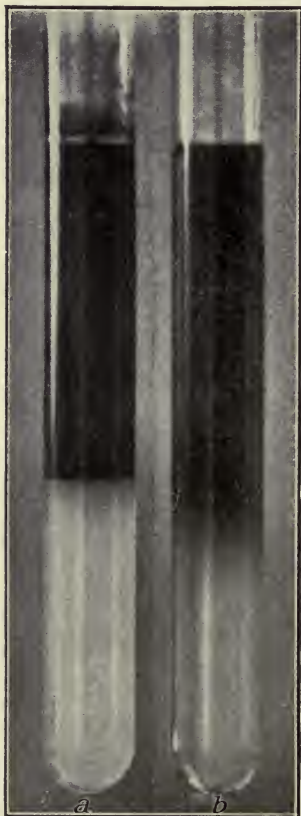
FIG. 1.—Diffusion of a colloid (a) and a "true" solution (b) into solid gelatin.
